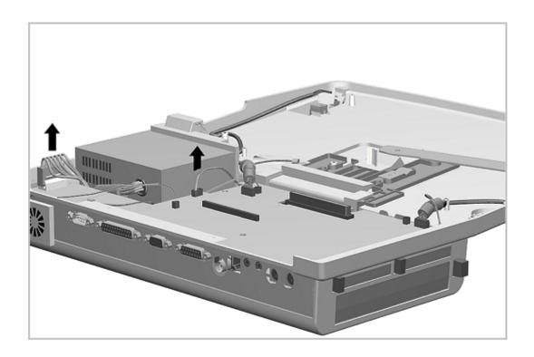
Figure 7-15. Disconnecting the Power Supply
